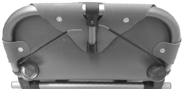
8. Mark the cable housing 2 1/2" (65mm) from one end, then slide that mark in the end over the cable end and into the hole in the shelf up to the mark. Repeat for the opposite side.
