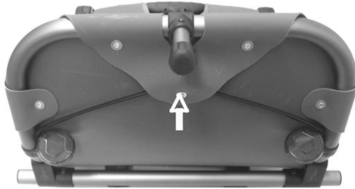
2. Pull cable out from under the flap on the lower side of the shelf. Cut cable on both sides of the ferrule.
