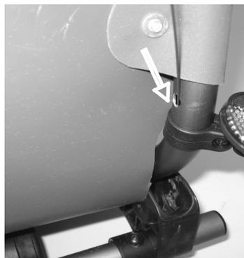
6. Thread the spring over the new cable, then hook the cable head into the plunger as shown. Insert the spring and plunger into the end of the shelf tube.
