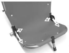
4. Remove then discard the cable. Keep the cable housing and plungers. Remove and retain the springs from inside of the shelf tube.
